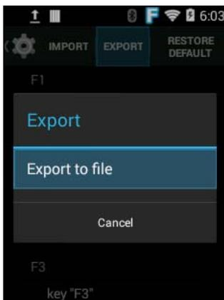
The Programmable Key configuration can be exported to a text file or imported into HT1.
